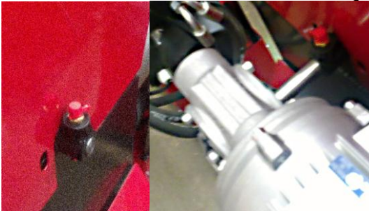
/The grease nipples are protected by red plastic dust caps./
